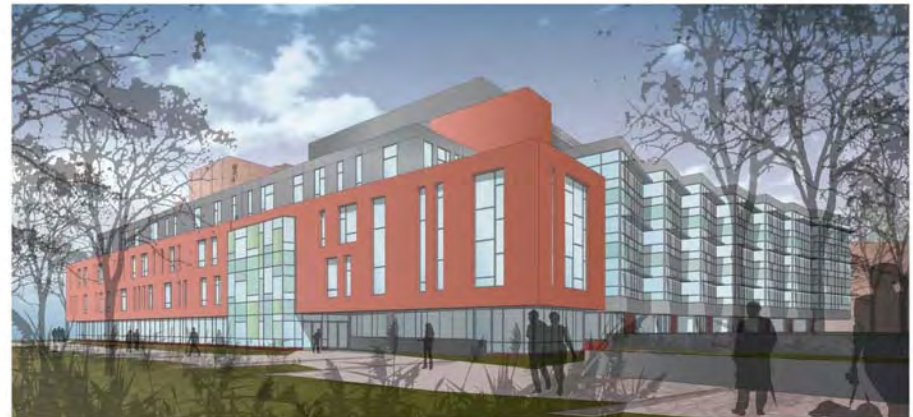
Brick Cladding Glazed Brick Cladding at First Floor Metal Panel Cladding Aluminum Framed Windows & Curtain Wall Existing Building
